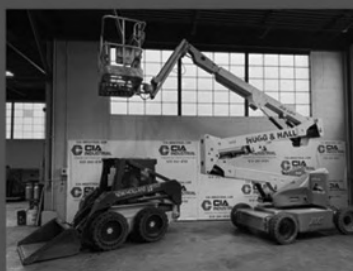
Skid Steer and Boom Lift
